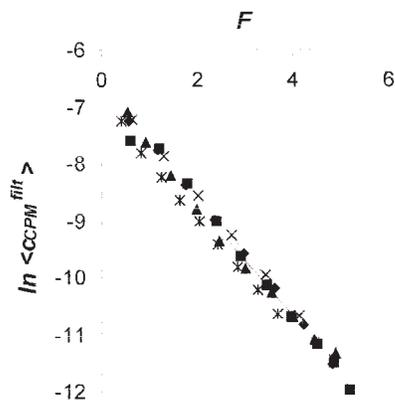
**Figure 3** Elution profiles of CPM in the presence of 0.13M NaCl: (◆) blank experiment, (■)  $\kappa$ -CAR, (▲)  $\iota$ -CAR, (×) ALG, (\*) CMC, and (—) linear tendencies. (See Table I for conditions and linear adjustments.)
